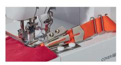
Dual function fold binder For making and attaching tapes in a finished size of 8mm width,
