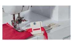
Bias tape binding set For folding and attaching 6mm or 12mm-wide bias tapes to fabric edge.
