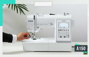
DROP IN A BOBBIN, THREAD IN THE DIRECTION OF THE ARROW AND YOU'RE READY TO SEW.
